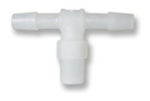
The AT-R Series are single-barbed by Male NPT threads Tee Adapters. Available in Black and Natural Nylon, Glass-Filled Nylon, Natural and White Polypropylene, PVDF, and Polyethylene that is NSF 51/61 listed. Thread sizes range from 1/8 inch to 1 inch. Barb sizes range from 1/4 inch to 1 inch.
