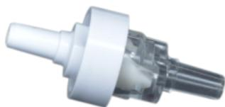
This is a non-barbed Acrylic or Polycarbonate Check Valve that has a Silicone duck bill. This is a normally open, one-way check valve. It prevents back flow leakage with minimal pressure. The ends of the ports measure .134 to accommodate 1/8" ID tubing. These fittings are also available with male and female Luer Locks.
