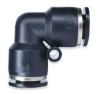
The PUE Series is a composite Union Elbow made of a PBT body and a Buna-N seal. The working pressure is 150 psi and a temperature range of  $32^{\circ}$  F to  $140^{\circ}$  F.
