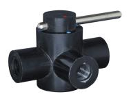
These ball valves are made of FDA Polypropylene with Viton® O-rings and 316 stainless steel handles. All connections are female NPT threaded. In addition, the pressure rating is 150 psi at 73°F. They are designed for use with liquid, gas, and vacuum applications. Inlet and outlet sizes are 1/8", 1/4", 3/8", 1/2", and 3/4". Also available in PVDF with actuation. Also, they are available in 2-way, 4-position 3-way, and 2-position 3-way orientations.
