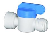
This Ball Valve is made of white Polypropylene with EPDM O-rings. It is a 1/4 turn from open to closed. Also, the maximum pressure is 150 psi and the temperature range is 33 F to 140 F. To be used with potable water, it is not suitable for inert gases or air. Furthermore, one end is male NPT threaded and the other end is a socket fitting.
