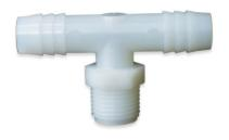
Male NPT thread by multi-barbed Tee Adapter is available in NSF-listed natural and black Nylon, NSF-listed black Polyethylene, and natural and black Polypropylene – both FDA-listed. Male NPT thread sizes are 1/8", 1/4", 3/8", 1/2", 3/4" and 1". The barb sizes available are 1/4", 3/8", 1/2", 3/4", 5/8" and 1".
