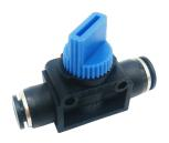
The HV Series Hand Valves are made with a PBT body, nickel-plated threads, and Buna-N O-rings. In addition, the valves can stop or reduce flow. The working pressure is 150 psi and the temperature range is  $32^{\circ}$  F to  $140^{\circ}$  F. They can be used for compressed air or inert gases.
