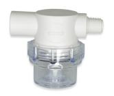
The PWF Series Plastic Bowl Filters have a Polypropylene or Nylon housing with a clear, profile 1-inch bowl filter. Available port sizes are 1/4 inch, 3/8 inch, and .170 inch barbs. Male and female NPT threads for these filters are 1/4 inch, 3/8 inch, and 1/2 inch. Available gaskets are EPDM, Viton®, and Buna-N. Filters: 20, 40, 80, 100, or 250 mesh 303 Stainless Steel; 5 and 70-micron Polyethylene screen; 10 Micron paper pleated screen.
