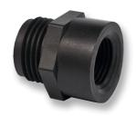
The MGHF Series is a Male garden hose by Female NPT threads garden hose fitting. Available FNPT thread sizes are 1/4 inch, 1/2 inch, and 3/4 inch. These fittings are available in either Nylon or Black Polypropylene.
