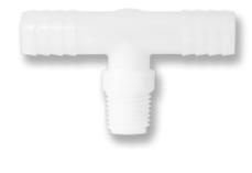
The AT series is an MNPT by plastic triple barbed tee adapter. It is molded of NSF listed Natural Nylon, Black Nylon, and Black Polyethylene. Optional materials are FDA listed Natural Polypropylene and Black Polypropylene. MNPT threads sizes are 1/8 inch, 1/4 inch, 3/8 inch, 1/2 inch, 3/4 inch, and 1 inch. The barb sizes available are 1/4 inch, 3/8 inch, 1/2 inch, 3/4 inch, 5/8 inch, and 1 inch.
