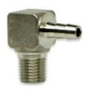
The SBHE Series is a 316 Stainless male NPT threads to barb  $90^{\circ}$  Elbow Adapter. Available MNPT thread sizes are 1/8 inch, 1/4 inch, 3/8 inch, and 1/2 inch. Available barb sizes are 1/4 inch, 3/8 inch, and 1/2 inch.
