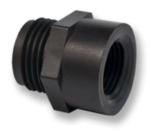
The MGHF Series is a Male garden hose by Female NPT threads garden hose fitting. Available FNPT thread sizes are 1/4 inch, 3/8 inch, 1/2 inch, 5/8 inch, and 3/4 inch. These fittings are available in either Nylon or Polypropylene.
