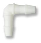
The EV Series are single barbed tube-to-tube elbows. These elbows are available in White and Black Nylon, Natural Polypropylene, Clear Polycarbonate, and PVDF. These elbows are available in equal or reducing sizes. Barb sizes are 1/16 inch, 1/8 inch, and 3/32 inch.
