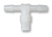
The AT-R Series are single-barbed by Male NPT threads Tee Adapters. Available in Black and Natural Nylon, Glass-Filled Nylon, Natural and White Polypropylene, PVDF, and Polyethylene that is NSF 51/61 listed. Thread sizes range from 1/8 inch to 1 inch. Barb sizes range from 1/4 inch to 1 inch.
