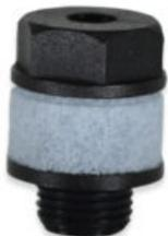
The NMP Series high-flow Muffler is made of Glass-Filled Nylon with a 40 micron sintered bronze screen. It is available with MNPT threads of 1/8 inch, 1/4 inch, and 3/8 inch. The maximum working pressure is 150 psi and the working temperature range is 35° F to 120° F.
