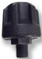
The MTM Series Muffler Breather is made of Glass-Filled Nylon. This series is available in 1/8 inch and 1/4 inch MNPT threads, both with a 10 micron element.
