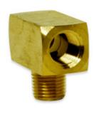
The BC Series are miniature Brass pipe fittings with various configurations of 10-32 inch UNF and 1/4-28 inch UNF male and female threads. These block fittings can be either female-to-female or male-to-female configurations of elbows, crosses, or tees.
