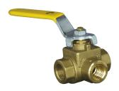
MBBV Series is a forged 3-way ball valve that offers flow options in both directions as well as allowing unimpeded flow when the handle is placed at a 45° angle. In addition, the temperature rating for this valve is 0-230°F. Also, the pressure rating of this ball valve is 600 WOG.
