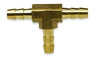
The BHT Series is a forged Brass multi-barbed Tee connector. Available barb sizes are 1/8 inch, 1/4 inch, and 3/4 inch. The working temperature range is -40° F to 160° F. Maximum working pressure is 150 psi. This fitting is designed for use with a hose clamp.
