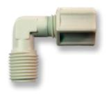
The CME Series are Male NPT Compression Fittings to an OD Elbow configuration. Use for Manifolds, Valves, Regulators, or mechanical instruments. They are molded of either Glass-Filled White Polylpropylene, NSF approved FDA approved Acetal for use with hot water applications, NSF approved FDA approved Nylon, or NSF approved FDA approved UV resistant PVDF. Provided with a poly gripper for use up to 220 psi. 1/8 inch units do not have a poly gripper.
