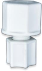
The CF Series Compression Female Pipe Threads, 1/8 inch to 1/2 inch, with compression fittings ranging from 1/4 inch to 5/8 inch tube connection without kinking attached tubing. Available in NSF approved Glass-Filled White Polypropylene, FDA and NSF approved Acetal (POM) for use with hot water applications, FDA and NSF approved Nylon, and UV resistant FDA and NSF rated PVDF. Provided with Poly gripper (except for 1/8 inch units) for us up to 220 psi.
