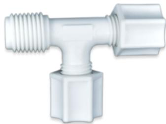
The CMR Series Male Thread Run with a compression connection on the branch. Male pipe threads are 1/8 inch to 3/4 inch. Compression Branch allows tubing connections of 1/4 inch to 7/8 inch without kinking attached tubing. Available in NSF approved Glass-Filled White Polypropylene, FDA and NSF approved Acetal (POM) for use with hot water applications, FDA and NSF approved Nylon, and UV resistant FDA and NSF rated PVDF. Provided with Poly gripper (except for 1/8 inch units) for us up to 220 psi.
