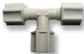
The CT Series Three port Compression Fittings are for 1/8 inch to 7/8 inch tubing connection without kinking attached tubing. Available in NSF approved Glass-Filled White Polypropylene, FDA and NSF approved Acetal (POM) for use with hot water applications, FDA and NSF approved Nylon, and UV resistant FDA and NSF rated PVDF. Provided with Poly gripper (except for 1/8 inch units) for use up to 220 psi. Available in a select number of reducing sizes.
