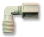
The CME Series are Male NPT Compression Fittings to an OD Elbow configuration. Use for Manifolds, Valves, Regulators, or mechanical instruments. They are molded of either Glass-Filled White Polylpropylene, NSF approved FDA approved Acetal for use with hot water applications, NSF approved FDA approved Nylon, or NSF approved FDA approved UV resistant PVDF. Provided with a poly gripper for use up to 220 psi. 1/8 inch units do not have a poly gripper.
