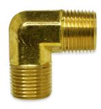
The BME Series is a 90° Brass forged Elbow, available in both equal and reducing sizes. Available Male NPT thread sizes are 1/8 inch, 1/4 inch, 3/8 inch, and 1/2 inch. The temperature range is -65° F to 250° F. The operating pressure is 1200 psi. They can be used for grease, fuels, refrigeration, and hydraulic applications. They meet ASA, ASME, and SAE specifications. Nickel-plated brass is available.
