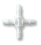
The CX Series is a standard single barbed Cross fitting with no molded parting line on the barb. The barb will expand the tubing to 50% above its normal size. It is available in White Nylon and Natural Polypropylene. The available equal barb sizes are 1/16 inch, 3/32 inch, and 1/8 inch. This cross-fitting is recommended for medical and laboratory environments.
