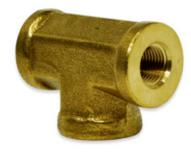
The BBFTR Series is a forged Brass female reducing Tee. The operating pressure for this tee is 1200 psi with a temperature range of -65° F to 250° F. The threads are Female NPT.
