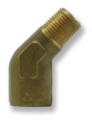
The BSE45 Series are 45° Brass Elbows available as both forged and barstock. The temperature range is -65° F to 250° F. The operating pressure is 1200 psi. They can be used for grease, fuels, refrigeration and hydraulic applications. They meet ASA, ASME and SAE specifications.
