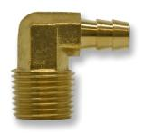
The BHME Series is a forged Brass multi-barbed  $90^{\circ}$  Elbow Adapter with male NPT threads. Available MNPT thread sizes range from 1/8 inch to 1 inch. In addition, available barb sizes range from 3/16 inches to 3/4 inches. Flow can be equal or reduced. The working temperature range is  $-40^{\circ}$  to  $160^{\circ}$  and the working pressure is 150 psi. Barstock is optional for some sizes (see list below).
