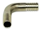
The SSES Series are 304 Stainless Steel  $90^{\circ}$  elbow hose barb splicer fittings. These elbows are intended to be used with hose clamps or similar clamps. Working temperatures are from -40° F to +160° F. Maximum working pressure is 150 psi. Available in barb sizes of 1/4 inch and 3/8 inch.
