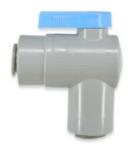
The EBV Series One-Way single direction Flow Ball Valve is made of PVC with standard Buna seals. Maximum pressure 125 psi and 140 degrees F and a thru hole of .437 used for air, water, gas, oxygen, and refrigeration applications. (not for vacuum)
