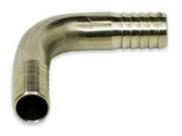
The SSES Series are 304 Stainless Steel  $90^{\circ}$  elbow hose barb splicer fittings. These elbows are intended to be used with hose clamp or similar clamps. Working temperatures are from -40° F to +160° F. Maximum working pressure is 150 psi. Available in barb sizes of 1/4 inch and 3/8 inch.
