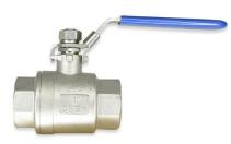
This two-way Brass Ball Valve has a pressure rating of 600 psi, and 150 psi is the working steam pressure. The maximum temperature is 366°F. The stem is blow-out proof, the ball is Chrome-plated Brass and the seat is PTFE. There is an adjustable screw packing nut. Both ports are equal in size and female NPT threads.
