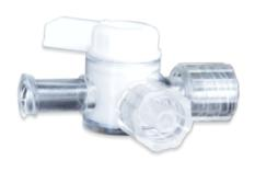
4-way Stopcock is available in Polycarbonate, Acetal, Polyethylene, HDPE, Acrylic and Silicone. These Stopcocks are chemically resistant and not made with DEHP. Connection options include male luer slip, male luer lock, male luer with spin lock, rotating male luer lock, female luer lock, and tubing ports. Psi is 50, higher pressures are available on request.
