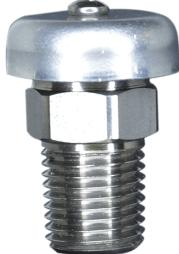
This is a vent-to-atmosphere Relief Valve. It is an accurate design that offers repeatability and dependability. Cracking pressure is set and tested for accuracy. Male NPT threads in 1/4", 3/8", and 1/2" sizes. Maximum pressure is 200 psi. Made of Nickel-plated Brass, 303 Stainless Steel and Brass. An optional dust cover is available.
