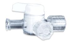
4-way Stopcock is available in Polycarbonate, Acetal, Polyethylene, HDPE, Acrylic and Silicone. These Stopcocks are chemically resistant and not made with DEHP. Connection options include male luer slip, male luer lock, male luer with spin lock, rotating male luer lock, female luer lock, and tubing ports. Psi is 50, higher pressures are available on request.
