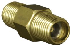
BLA Ball check valves. Brass and 303 Stainless Steel bodies in three sizes: 10-32 Unf Female, 1/8 MNPT, and 1/4 MNPT.
