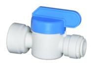
This Ball Valve is made of white Polypropylene with EPDM O-rings. It is a 1/4 turn from open to closed. The maximum pressure is 150 psi and the temperature range is 33 F to 140 F. To be used with potable water, it is not suitable for inert gases or air. One end is male NPT threaded and the other end is a socket fitting.
