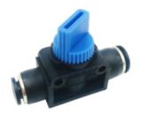
These Hand Valves are made with a PBT body, nickel-plated threads, and Buna-N O-rings. The valves can stop or reduce flow. The working pressure is 150 psi and the temperature range is  $32^{\circ}$  F to  $140^{\circ}$  F. They can be used for compressed air or inert gases.
