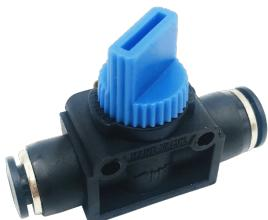
The HV Series Hand Valves are made with a PBT body, nickel-plated threads, and Buna-N O-rings. In addition, the valves can stop or reduce flow. The working pressure is 150 psi and the temperature range is 32° F to 140° F. They can be used for compressed air or inert gases.
