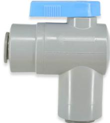
The EBV Series One-Way single-direction Flow Ball Valve is made of PVC with standard Buna seals. Maximum pressure 125 psi and 140 degrees F and a thru-hole of .437 used for air, water, gas, oxygen, and refrigeration applications. (not for vacuum)
