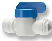
The PKV Series is a Polypropylene Ball Valve with Push-to-Connect connections and EPDM seals. Not suitable for vacuum, air, or inert gases.
