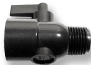
The LRH Series Two-Way Ball Valves are made from PVC or ABS plastic with a 7 CV Flow and 125 psi with Buna seals standard. (one-way valve is optional)
