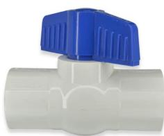
The BRS Series compact PVC quarter-turn shut-off Ball Valves with PTFE sets and EPDM O-ring seals are used in industrial and plumbing applications. Available in schedule 80 (gray) and schedule 40 (white). Sizes range from ½ inch to 2 inches.
