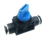
The HV Series Hand Valves are made with a PBT body, nickel-plated threads, and Buna-N O-rings. In addition, the valves can stop or reduce flow. The working pressure is 150 psi and the temperature range is 32° F to 140° F. They can be used for compressed air or inert gases.
