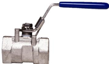
The MSBV Series Ball Valves have a Stainless Steel body, ball, stem, and insert with an 800 psi WOG and PTFE thrust washer. 304 Stainless Steel locking handle. Full ported 1000 psi WoG 2 piece version up to 2-inch Female NPT available.
