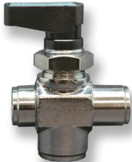
AMS Series Ball Valves available in inline, elbows, and 3-way tee configurations, are Chrome Plated Brass with female NPT, male NPT, and Push-to-Connect ports. They all have a temperature range of 0° F to 175° F and are recommended for air, oil, water, and gas use.
