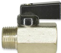
This is a Chrome-plated Forged Brass Mini Ball Valve with a Chrome-plated Brass ball. The maximum working pressure is 450 psi, 142 psi at 356°F, and 355 psi at 212°F. Available in female by female and male by female. Available with a flag handle, a lever handle, or a tee handle, or can be adjusted with a screwdriver.
