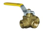
This forged 3-way ball valve offers flow options in both directions as well as allowing unimpeded flow when the handle is placed at a 45° angle. The temperature rating for this valve is 0-230°F. The pressure rating of this ball valve is 600 WOG.
