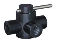
These ball valves are made of FDA Polypropylene with Viton® O-rings and 316 stainless steel handles. All connections are female NPT threaded. The pressure rating is 150 psi at 73°F. They are designed for use with liquid, gas, and vacuum applications. Inlet and outlet sizes are 1/8", 1/4", 3/8", 1/2", and 3/4". Also available in PVDF with actuation. They are available in 2-way, 4-position 3-way, and 2-position 3-way orientations.
