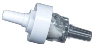
This is a non-barbed **Acrylic or Polycarbonate Check Valve** with a Silicone duck bill. This is a normally open, one-way check valve. It prevents backflow leakage with minimal pressure. The ends of the ports measure .134 to accommodate 1/8" ID tubing. These fittings are also available with male and female Luer Locks.
