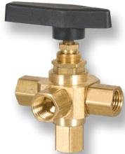
The BSL Series are Detent Panel Mount 5-Way Ball Valves in 10-32, 1/8 inch Female NPT, 1/4 inch Female NPT, 1/8 inch Male NPT, or 1/4 inch Male NPT with EPDM seals and 500 psi.
