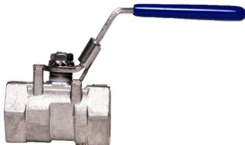
The MSBV Series Ball Valves have a Stainless Steel body, ball, stem, and insert with an 800 psi WOG and PTFE thrust washer. 304 Stainless Steel locking handle. Full ported 1000 psi WoG 2 piece version up to 2-inch Female NPT available.
