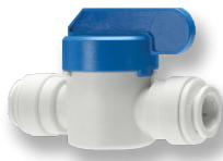
The PKV Series is a Polypropylene Ball Valve with Push-to-Connect connections and EPDM seals. Not suitable for vacuum, air, or inert gases.
