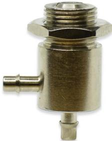
Nickel Plated Panel Mount Needle Valve with a 3° pin angle, 64 TPI for fine adjustment. Buna-N seal standard and it has a screwdriver slot for easy adjustment. Operating temperature -40° F to 200° F. The recommended filtration is 5 microns. Barbed fittings for flexible tubing.
