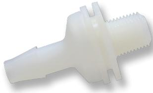
The CMKV Series Plastic Check Valves are 1/8 inch Male NPT by Barb sizes of 1/8 inch, 3/16 inch, 1/4 inch, and 3/8 inch. The flow is from thread to barb. Material / Disc combinations are available in PVDF with FKM, Polypropylene with FKM, Polycarbonate with Neoprene, Polycarbonate with Silicone, Nylon with Silicone, and Nylon with Neoprene.
