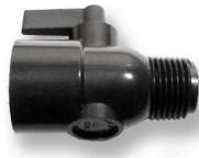
The LRH Series Two-Way Ball Valves are made from PVC or ABS plastic with a 7 CV Flow and 125 psi with Buna seals standard. (one-way valve is optional)
