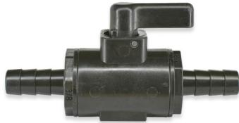
The PJV Series Micro Ball Valves are of Polypropylene and reinforced fiberglass with a 90-degree rotating handle and FKM O-rings. The standard pressure is 150 psi with a maximum temperature of 150° with a maximum pressure of 300 psi at 70° F.
