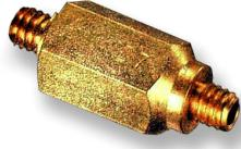
The CLCV Series Brass Check Valves have 10-32 inch ports, a Nitrile seal, and a Stainless Steel spring. It permits flow in only one direction and is used for air and hydraulics. The input psi is 300 maximum. The crack pressure is 1/2 psi and the temperature range is 32° F to 230° F. The 1/8-inch valve has a maximum input pressure of 1000 psi. Otherwise, all other attributes are the same as the 10-32 inch valve.
