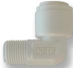
The DCE Series is a rigid male Check Valve elbow made of Acetal that is NSF 51® certified and meets NSF 61® requirements. The available male threads are 1/8 inch, 1/4 inch, and 3/8 inch. OD tubing sizes are 5/32 inch, 3/16 inch, 1/4 inch, 5/16 inch, 3/8 inch, and 1/2 inch. The working pressure at 77° F is 232 psi, and at 158° F it is 145 psi. The working temperature range is from 32° F to 158° F. It can be used for compressed air, inert gases, water, and other fluids.
