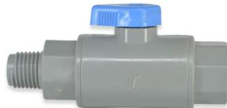
The EBV Series One-Way single-direction Flow 90-degree Ball Valve is made of PVC with standard Buna seals. Maximum pressure 125 psi and 140 degrees F and a thru-hole of .437 used for air, water, gas, oxygen, and refrigeration applications. (not for vacuum)
