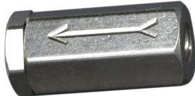
The NCV Series Nickel-Plated Brass Poppet Check Valve has options of Buna-N, EPDM or FKM seals. The operating pressure is 0 to 125 psi and the flow rate ranges from 2.5 to 9.5 scfm. Input and output port sizes are 10-32 inch UNF and 1/16 inch Barb.
