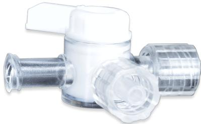
4-way Stopcock is available in Polycarbonate, Acetal, Polyethylene, HDPE, Acrylic and Silicone. These Stopcocks are chemically resistant and not made with DEHP. Connection options include male luer slip, male luer lock, male luer with spin lock, rotating male luer lock, female luer lock, and tubing ports. Psi is 50, higher pressures are available on request.
