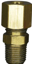
The CMCV Series Brass Ball Check Valves are compression fittings. This series has Tube OD of 1/8 inch, 1/4 inch, and 3/8 inch. Male NPT thread sizes of 1/8 inch and 1/4 inch are available. The working pressure for the 1/8 inch tube OD is 400 psi, for the 1/4 inch it is 300 psi, and for the 3/8 inch, it is 200 psi. The temperature range is -65° F to 250° F at maximum operating pressures.
