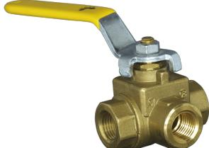
MBBV Series is a forged 3-way ball valve that offers flow options in both directions as well as allowing unimpeded flow when the handle is placed at a 45° angle. In addition, the temperature rating for this valve is 0-230°F. Also, the pressure rating of this ball valve is 600 WOG.
