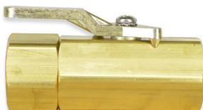
This is a Solid Chrome plated Brass Mini Ball Valve. This valve works in both directions because of a double seal system. It has a blow-out-proof Brass stem. The 1/4 turn handle has a mechanical stop. The maximum working pressure is 235 psi but will handle 300 psi at 75°F. The temperature range is 32°F to 176°F. Available in female by female and male by female. *\*\*\*This product is not lead-free.\*\*\**
