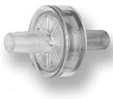
The BBCV Series Check Valve has a Male Slip Luer with 30 psi back pressure and 1/4 psi inlet cracking pressure. This series comes in ABS or Polycarbonate housing, both with Silicone Discs.
