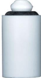
These Cartridge Insert Valves can be installed into tubing lines or glued into manifolds. The optional housing materials are Nylon, Polypropylene, Acrylic, Acetal, PVDF, and Polycarbonate. Springs are 316 Stainless Steel or Hastelloy® (1/2 psi). O-Rings are of Buna-N, EPDM, FKM, Silicone and Kalrez. Available sizes are 1/4", 5/16", 3/8", 1/2", 5/8" and 3/4" OD. Standard crack pressure for all valves except 3/4" OD is 3" H<sub>2</sub>O 0.1 psi, 5 psi, or 1.5 psi.
