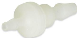
These ASD Series single barbed enlarging duckbill Check Valves are available in several materials such as Nylon (N), Polypropylene (PP), or Polycarbonate (PC) housing. These Check Valves have a Silicone diaphragm. The available barb sizes are 1/8 inch by 3/16 inch and 3/16 inch by 1/8 inch.
