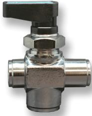
AMS Series Ball Valves available in inline, elbows, and 3-way tee configurations, are Chrome Plated Brass with female NPT, male NPT, and Push-to-Connect ports. They all have a temperature range of 0° F to 175° F and are recommended for air, oil, water, and gas use.
