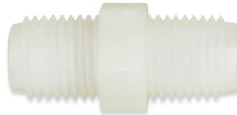
The CVK Series are male-by-male Check Valves made of natural PVDF. It has a 316 Stainless Steel spring and ball Viton® O-ring. Other O-ring options are EPDM and Fluorosilicone (blue). These check valves have a 1-2.5 psi cracking pressure with a maximum operating pressure of 220 psi and a maximum working temperature of 180°F. Available with a Hastelloy® spring and PTFE ball. Available Male NPT thread sizes are: 1/8 inch, 1/4 inch, 3/8 inch, and 1/2 inch.
