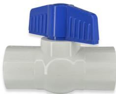
The BRS Series compact PVC quarter-turn shut-off Ball Valves with PTFE sets and EPDM O-ring seals are used in industrial and plumbing applications. Available in schedule 80 (gray) and schedule 40 (white). Sizes range from 1/2 inch to 2 inches.
