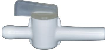
This is a miniature stopcock made of high-density polypropylene. The key turns easily so no lubricant is needed, eliminating blockage of the bores with grease. This is not for pressurized lines.
