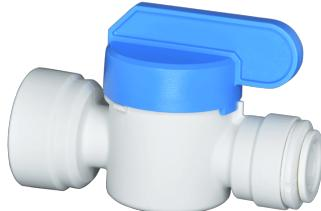
This Ball Valve is made of white Polypropylene with EPDM O-rings. It is a 1/4 turn from open to closed. Also, the maximum pressure is 150 psi and the temperature range is 33 F to 140 F. To be used with potable water, it is not suitable for inert gases or air. Furthermore, one end is male NPT threaded and the other end is a socket fitting.
