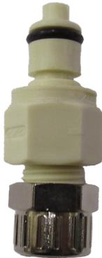
40AC Insert is designed with a reliable compression fitting, making it suitable for both 1/4 inch and 3/8-inch OD Poly Tubing. This insert features a nickel-plated nut, which enhances its durability and resistance to corrosion. The robust construction ensures a secure and leak-free connection, making it ideal for various applications requiring high performance and reliability.
