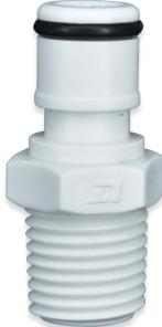
50AC Quick Coupler Acetal Fitting Threaded Inserts, Two thread sizes available, 1/4 and 3/8 NPT. For use with the all 50 series female couplers.
