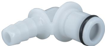
The 20AC PB4 Series is a Male Quick Coupler with a 1/8 Flow and a 90° Elbow. This product is made from Acetal with a Buna O-ring. Also, the available barb sizes are 1/8 and 1/4 with or without shutoff.
