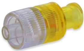
The QCD Series Luer Check Valves are made of Polycarbonate and have a Silicone duck bill. The low cracking pressure is 0.433 psi, which determines when the component starts to open. The OD sizes are 5/64 inch, 7/64 inch, and 9/64 inch. Also available with female and male Luer Locks.
