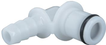
The Quick Coupler Male features a 1/4 flow 90-degree elbow design, crafted with a durable Acetal body and a Buna O-ring for reliable sealing. This versatile coupler is available with either a 1/4 inch or 3/8 inch barb, providing flexibility for various applications. Additionally, it can be supplied with or without a shutoff mechanism, catering to different operational needs.
