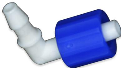
Male slip luer by barb Elbow. The barb accommodates 3/32" ID tubing. This luer may be used with a separate rotating lock ring. It is available in white and black Nylon, black Polypropylene, and clear Polycarbonate.
