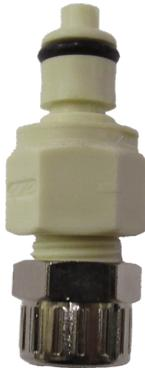
40AC Insert is designed with a reliable compression fitting, making it suitable for both 1/4 inch and 3/8-inch OD Poly Tubing. This insert features a nickel-plated nut, which enhances its durability and resistance to corrosion. The robust construction ensures a secure and leak-free connection, making it ideal for various applications requiring high performance and reliability.
