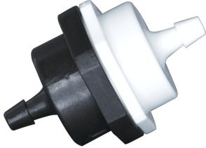
This check valve is made of either white polypropylene, natural Nylon, or black or natural Kynar®. It is available with a Buna-N, EPDM, or Viton® seal. It has a 302 stainless steel spring. The cracking pressure is .25 or 1 psi. The maximum pressure is 125 psi and the maximum operating temperature is 140°F. The ports can be single or multi-barbed.
