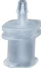
The FSL & MSL Series is a Male and Female Slip Luers in clear ABS, white Nylon, clear Polycarbonate, PVDF, and radiation-stable polycarbonate. Barb sizes range from 1/16" to 1/4". 1/4-28 male UNF threads are also available.
