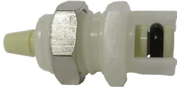
1/16 Flow Panel Mount Insert, 7/16-24 UNF thread for 1/2 ID thru hole.
