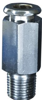
QCS Series has a 316 Stainless Steel Coupler body with a Male NPT threaded connection to a Push-to-Connect stem. Also, the OD sizes are 1/4" and 3/8" and the male threads sizes are 1/8" and 1/4". The temperature range is from 0° F to 150° F. The maximum working pressure is 150 psi. Furthermore, the coupler works well with Polyethylene, Nylon, Polypropylene, or Vinyl Tubing. This coupler is also available in chrome-plated brass.
