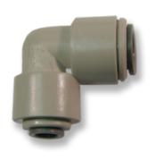
Push-to-Connect Elbow connectors available in Acetal, Polypropylene, and Kynar°® used to join tubing of Polyethylene, Brass, or Copper. Sizes range from 5/32 inch OD to 1/2 inch OD including reducing sizes. Gray or White Acetal are NSF and FDA approved and have Buna seals for use in air, gases, and potable water applications. White Polypropylene with EPDM seals or PVDF with FKM seals. Maximum temperature 140°F at 60 psi for Polypropylene.
