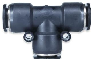
The PUT Series is a Union Tee Fitting that has 3 push-to-connect ports of equal sizes. The body is PBT resin. In addition, the working pressure is 150 psi and the temperature range is 32° F to 140° F. For use with compressed air and inert gases.
