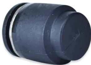
The PPF Series is a push-to-connect cap for use with all push-to-connect fittings to block a port. The body is PBT with a Buna-N O-Ring. This fitting is also available in metric sizes.
