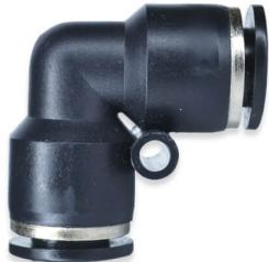
The PUE Series is a composite Union Elbow made of a PBT body and a Buna-N seal. The working pressure is 150 psi and a temperature range of 32° F to 140° F.
