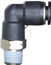
Push-to-connect fitting is a male compact Swivel Elbow with a hex configuration. Working pressure 150 psi, the temperature range is 32° F to 140° F. Nickel Plated Brass, Buna-N O-ring, and the grip ring is Stainless Steel. For use with compressed air and inert gases. Long stem version available. SAE and G threads have an O-ring below the hex.
