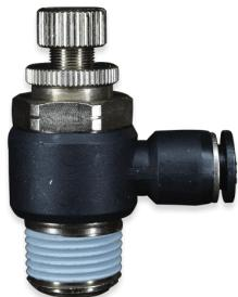
DEFV series is a Push-to-Connect Flow Control Valve Elbow made with nickel-plated threads and a stem with a PBT body. Standard controls flow out but checks the flow back. Also, these valves needle the flow from the tube and check the flow back through the tubing line. They are equipped with a single push-to-connect port at a 90° angle to the male thread. Furthermore, thread sizes are 10-32, 1/8", 1/4", 3/8" and 1/2".
