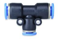
Union Tee fitting with 2 push-to-connect ports of equal sizes and 1 push-to-connect port that is a reducer located  $90^\circ$  apart. The body is PBT resin. The working pressure is 150 psi and the temperature range is  $32^\circ$  F to  $140^\circ$  F. For use with compressed air and inert gases.
