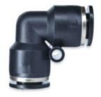
Composite Union Elbow made of a PBT body and a Buna-N seal. The working pressure is 150 psi and a temperature range of  $32^{\circ}$  F to  $140^{\circ}$  F.
