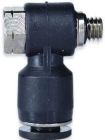
Push-to-connect adjustable male swivel 90° Elbow with NPT and UNF threads. The working pressure is 150 psi, and the temperature range is 32° F to 140° F. This series is made of PBT resin, nickel-plated brass with a Buna-N O-ring, and a Stainless Steel grip ring. For use with compressed air and inert gases. This fitting is also available in metric sizes. In fact, these fittings can swivel a full 360°.
