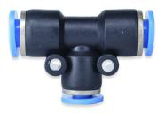
Union Tee fitting with 2 push-to-connect ports of equal sizes and 1 push-to-connect port that is a reducer located 90° apart. The body is PBT resin. The working pressure is 150 psi and the temperature range is 32° F to 140° F. For use with compressed air and inert gases.
