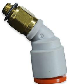
The PEM45 Series is a male push-to-connect fitting configured with a 45° elbow. The working pressure is 150 psi and the temperature range is 32° F to 140° F. Also, the metal body material is Nickel-plated Brass and the resin is PBT. This product is intended for use with compressed air and inert gases.
