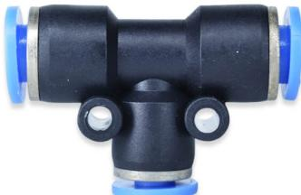
Union Tee fitting with 2 push-to-connect ports of equal sizes and 1 push-to-connect port that is a reducer located 90° apart. The body is PBT resin. The working pressure is 150 psi and the temperature range is 32° F to 140° F. For use with compressed air and inert gases.
