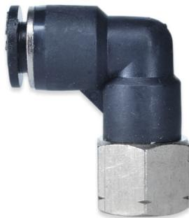
The PEFC Series is a push-to-connect Swivel Female Elbow that is configured with a 90° body **with an external hex for tightening**. The working pressure is 150 psi and the temperature range is 32° F to 140° F. Metal body material is Nickel-Plated Brass and the resin is PBT. For use with compressed air and inert gases.
