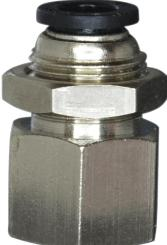
Push-to-connect female Bulkhead Union fitting with female NPT and BSPT threads. It is made of nickel-plated brass with PBT resin. The working pressure is 150 psi and the temperature range is 32° F to 140° F. It can be used with compressed air and inert gases.
