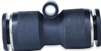
Compact Straight Fitting with two push-to-connect ports in opposite directions. The body is PBT resin. The working pressure is 150 psi and the temperature range is 32° F to 140° F. Suitable for applications involving compressed air and inert gases.
