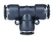
The PUT Series is a Union Tee Fitting that has 3 push-to-connect ports of equal sizes. The body is PBT resin. In addition, the working pressure is 150 psi and the temperature range is 32° F to 140° F. For use with compressed air and inert gases.
