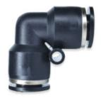
Composite Union Elbow made of a PBT body and a Buna-N seal. The working pressure is 150 psi and a temperature range of 32° F to 140° F.
