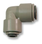
Push-to-Connect Elbow connectors available in Acetal, Polypropylene, and Kynar<sup>®</sup> used to join tubing of Polyethylene, Brass, or Copper. Sizes range from 5/32 inch OD to 1/2 inch OD including reducing sizes. Gray or White Acetal are NSF and FDA approved and have Buna seals for use in air, gases, and potable water applications. White Polypropylene with EPDM seals or PVDF with FKM seals. Maximum temperature 140°F at 60 psi for Polypropylene.
