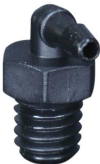
The AL-S Series is a male UNF threaded elbow adapter and is available in White and Black Nylon, Natural and Black Polypropylene, and Natural PVDF. Available in 10-32 inch UNF straight and tapered threads, and the barb sizes are 1/16 inch, 3/32 inch, and 1/8 inch.
