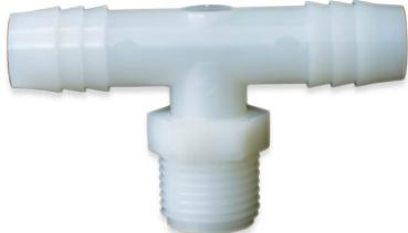
Male NPT thread by multi-barbed Tee Adapter is available in NSF-listed natural and black Nylon, NSF-listed black Polyethylene, and natural and black Polypropylene – both FDA-listed. Male NPT thread sizes are 1/8", 1/4", 3/8", 1/2", 3/4" and 1". The barb sizes available are 1/4", 3/8", 1/2", 3/4", 5/8" and 1".
