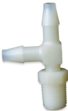
The MR-I Series is a industrial grade male run Tee Adapter made in natural Nylon and Polypropylene. The NPT thread sizes are 1/8" and the equal barbs are 1/8" and 3/16".
