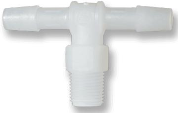
The AT-R Series are single-barbed by Male NPT threads Tee Adapters. Available in Black and Natural Nylon, Glass-Filled Nylon, Natural and White Polypropylene, PVDF, and Polyethylene that is NSF 51/61 listed. Thread sizes range from 1/8 inch to 1 inch. Barb sizes range from 1/4 inch to 1 inch.
