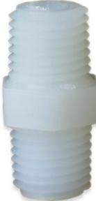
The HN-R Series is a male-by-male NPT Hex Nipple and Hex Nipple reducer. It comes in Natural, Black, and Glass-Filled Black Nylon, Natural Polypropylene, Gray PVDF, and Polyethylene. The Polyethylene is certified NSF 51/61. Available sizes range from 1/8 inch to 1 inch.
