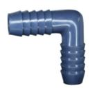
This Elbow adapter is made of PVC and can be used for irrigation and O.E.M applications. There is a wide variety of configurations available for use with Polyethylene pipe sizes 1/2" through 2". It conforms to ASTM D 2609 and is NSF certified for use with potable water. Female NPT thread sizes are 1/2", 3/4", 1", 1-1/4", 1-1/2" and 2". Barb sizes range from 1/2" to 1-1/2".
