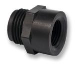
The MGHF Series connects male garden hose threads to female NPT fittings for secure, leak-free performance. Available in 1/4", 1/2", and 3/4" FNPT sizes, it's made from durable Nylon or Black Polypropylene for long-lasting strength and chemical resistance.
