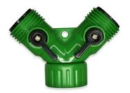
The dual Garden Hose Shutoff swivel has an ABS body, ball, and handle. It has a Zinc plated steel screw and Buna-N seal. It flows from female to male. Shutoffs are designed for city water pressure to a maximum of 80 psi.
