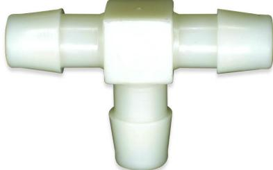
The T-I Series is a standard equal barb Tee made of white Nylon and natural Polypropylene. It is available in 1/16", 1/8" and 3/16" barbs.
