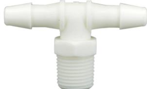
AT-S Series is an Adapter Tee available in black and white Nylon, black Polypropylene, and PVDF. There is straight male 10-32 UNF threads, male 1/8" NPT threads, and tapered 10-32 UNF threads. The barb sizes are 1/16" 3/32", 1/8", 3/16", and 1/4".
