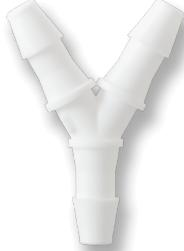
Y-S Series Wye tube fitting has equal single barbs and works well with flexible tubing. The barbs can expand tubing up to 50% above its normal size. This allows higher pressure capabilities. Available materials are White and Black Nylon, Natural Polypropylene, Polycarbonate, and PVDF. Barb sizes are 1/16 inch, 3/32 inch, 1/18 inch, 5/32 inch, 3/16 inch, and 1/4 inch. These Wyes are used primarily in laboratory and medical environments.
