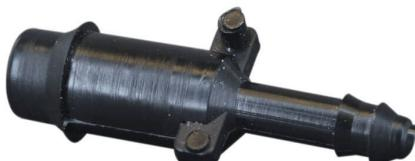
The VC-S Series are straight vacuum connectors in equal and reducing styles. It is made of Natural or Black Nylon 6/6. Equal barb sizes are 1/8 inch, 3/16 inch, 1/4 inch, 5/16 inch, 3/8 inch, 1/2 inch, and 5/8 inch. In addition, reducing barb sizes are 3/16 inch by 5/32 inch, 1/4 inch by 1/8 inch, 1/4 inch by 3/16 inch, 5/16 inch by 1/4 inch, and 3/8 inch by 1/4 inch. The working temperature range is -20° F to 212° F. These connectors are used for air, liquid, and vapor applications.
