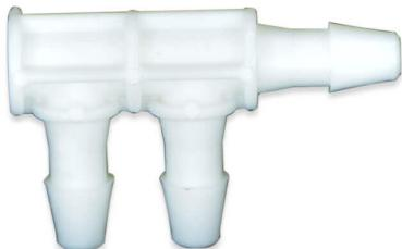
The DTF-S Series is a three-port F-style fitting usually used with flexible tubing. It can expand tubing by 50% of its normal ID. This permits high-pressure capabilities. This fitting is available in White Nylon and Natural Polypropylene. All three ports are equal. Available barb sizes are 1/16 inch, 3/32 inch, and 1/8 inch.
