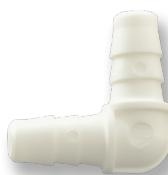
The L-IG Series are multi-barbed elbows made of Black and White Nylon and Gray Polypropylene. The ports are 1/16 inch and 1/8 inch. The maximum working pressure is 125 psi and the temperature ranges are: Nylon -50° F to 180° F; Polypropylene -40° F to 200° F.
