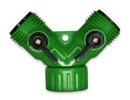
The 5114S Series is a durable and efficient dual garden hose shutoff swivel, designed for smooth water control. Crafted with a sturdy ABS body, ball, and handle, it ensures reliable performance. The shutoff features a zinc-plated steel screw and a high-quality Buna-N seal for enhanced durability. Designed to accommodate city water pressure up to a maximum of 80 psi, it allows seamless water flow from female to male connections.
