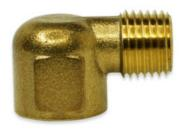
The BSTE Series are 90° Brass Street Elbows, available as both forged and barstock. The barstock fitting is available in a short version. The forged is available as a reducer. Available MNPT and FNPT thread sizes are 1/8 inch, 1/4 inch, 3/8 inch, 1/2 inch, and 3/4 inch. The temperature range is -65° F to 250° F. The operating pressure is 1200 psi. They can be used for grease, fuels, refrigeration and hydraulic applications. They meet ASA, ASME and SAE specifications.
