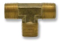
The BMT Series is a male forged Brass Tee Connector. Available male NPT thread sizes are 1/8 inch, 1/4 inch, 3/8 inch, and 1/2 inch. All sizes are also available in nickel-plate.
