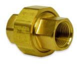
The FXF Series is a Brass female-by-female union. The brass fittings are available in four sizes, the nickel plated in five sizes, as noted below. The maximum operating pressure is 1200 psi and the working temperature range is -65° F to 250° F.
