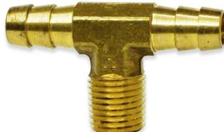
The BHMT Series is a Brass Tee. The size available is 1/4" male NPT threads to 3/8" barb. In addition, the maximum pressure for this Tee is 150 psi and the temperature range is -40° F to 160° F. This product is designed to be used with hose clamps.
