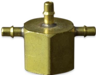
The FAT Series are Brass female adapters with bite-style barbs. Any different Barb size can be placed on any hex. FNPT thread sizes available for this series are 1/8 inch and 1/4 inch. Barb sizes range from 5/64 inch to 3/8 inch.
