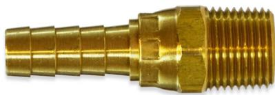
The BHAS Series is a long Brass Swivel with male NPT threads to hose barbs. The maximum working pressure is 150 psi at -40° F to 160° F.
