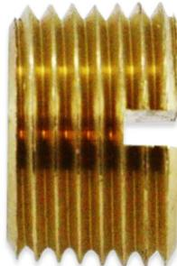
BSLP Series is a brass slotted head Plug with NPT threads. The working pressure is 1200 psi and the temperature range is -65° F to 250° F. It is ASA, ASME, and SAE compliant. Nickel plated is available.
