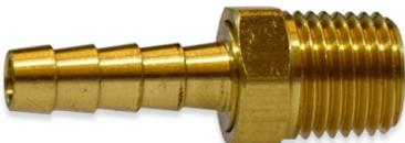
The SSWS Series is a Brass Swivel Adapter. It is available with male NPT threads to female NPT threads or a barb connection. The working pressure for both the threaded and barbed swivels is 300 psi. Both swivels have a bronze thrust bearing and EPDM or FKM seals. This swivel provides a full 360° rotation. The barbs are intended to be used with a hose clamp.
