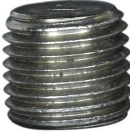
HCSS Series is a Bar stock Hex Socket Plug made of 304 or 316 Stainless Steel. It can be used with air, water, oil, natural gas or steam. Also, the maximum pressure is 300 psi at 72° F or 150 psi at 366 ° F for steam.
