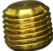
The BPC Series is a Brass recessed hex Plug with male NPT threads. The working pressure is 1200 psi and the temperature range is -65° F to 250° F. It is ASA, ASME, and SAE compliant.
