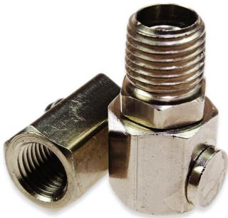
Nickel-plated brass Orbital Swivel connector with male-to-male, male-to-female, and female-to-female NPT threads with a full range of motion. The fittings swivel at the pipe threads and between the segments.
