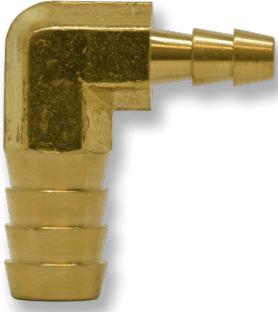
The BHBE Series is a forged Brass multi-barbed 90° Elbow connector. Barb sizes range from 1/8 inch to 1/2 inch. The working temperature range is -40° F to 160° F. Maximum pressure rating is 150 psi. This fitting is designed to be used with a hose clamp.
