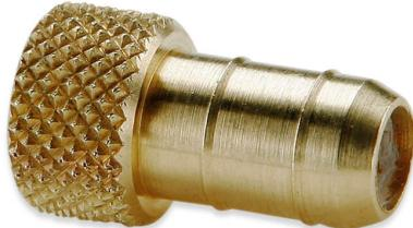
The DTP Series is a brass barbed tube plug. This fitting has excellent vibration resistance and requires no clamp. The maximum working pressure is 150 psi and the temperature range is -65° F to 90° F. This fitting can be used in humidifiers, pneumatic systems, and filters.
