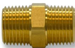
This is a brass-close Hex Nipple with male NPT threads. The pressure rating for this piece is 1200 psi. It can be used for fuels, grease, refrigeration, and hydraulic systems. Some sizes are available in nickel plates.
