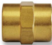
Brass connector with equal female NPT threads. The pressure rating for this connector is 1200 psi and the temperature range is -65° F to 250° F. It meets the specifications for ASA, ASMER, and SAE.
