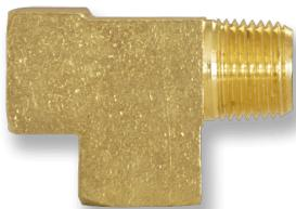
The STM Series is a male-run street tee available in forged or bar stock Brass. The temperature range for these tees is -65° F to 250° F. The working pressure is 1200 psi. These are ASA, ASME, and SAE compliant. Nickel-Plate is available in some sizes.
