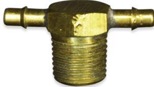
The MT Series are Brass male Tee adapters with bite-style barbs. Available male NPT thread sizes range from 1/16 inch to 1/4 inch and the available barb sizes range from 1/16 inch to 1/2 inch.
