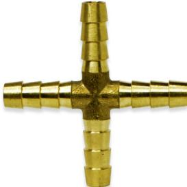
This series of Brass connectors is composed of straight connectors, elbows, tees, and crosses. The working temperature range is -40° F to 160° F. The straights, tees, and crosses have equal barb sizes. The elbows are both equal and reducing. These fittings are designed for use with hose clamps.
