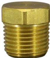
The BHP Series is a Brass hollow-core Hex Plug. These plugs come in Male NPT thread sizes of 1/8 inch, 1/4 inch, 3/8 inch, 1/2 inch, 3/4 inch, and 1 inch. The temperature range for this plug is -65° F to 250° F and has a pressure rating of 1200 psi. This plug is also available in Nickel-Plate and Stainless Steel.
