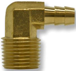
The BHME Series is a forged Brass multi-barbed 90° Elbow Adapter with male NPT threads. Available MNPT thread sizes range from 1/8 inch to 1 inch. In addition, available barb sizes range from 3/16 inches to 3/4 inches. Flow can be equal or reduced. The working temperature range is -40° to 160° and the working pressure is 150 psi. Barstock is optional for some sizes (see list below).
