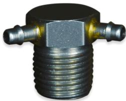
The MEV Series are brass MNPT thread with bite-style barbs at 60 degree to the flats. These elbows come in 3 different sizes of the angle between elbows - 60°, 90° and 120°. This series comes in MNPT thread sizes ranging from 1/8 inch to 3/8 inch and barb sizes ranging from 1/16 inch to 1/2 inch. Also available in Nickel-Plated Brass and 303 Stainless Steel.
