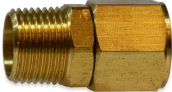
The SNPW Series is an Inline Brass Swivel connector with female to male NPT threads. The swivel allows for a full 360° rotation. Also it has Buna-N or FKM O-rings with a Polyphenylene thrust bearing.
