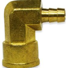
The BHFE Series is a Brass 90° Elbow, Female NPT threads to multi-barb Adapter. Available FNPT sizes are 1/8 inch, 1/4 inch, and 3/8 inch. Available barb sizes are 1/4 inch, 5/16 inch, 3/8 inch, and 1/2 inch. The temperature range is -40° F to 160° F. The maximum working pressure is 150 psi. This fitting is intended for use with a hose clamp.
