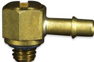
The CAE Series are Brass 10-32 inch UNF by bite-style single barb adjustable fitting with slotted adjustment flush to the surface. Elbow and Tee configurations. Also available in Nickel-Plated.
