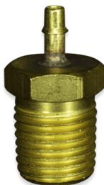
The DMA Series a Brass male NPT thread to ID bite-style barb adapter that works well with Polyethylene tubing. This fitting has excellent vibration resistance and requires no clamp. The maximum working pressure is 150 psi and the temperature range is -65° F to 90° F. Available MNPT thread sizes are 1/16 inch, 1/8 inch, 3/8 inch, 1/4 inch, and 1/2 inch. ID sizes range from .170 inch to .375 inch.
