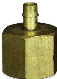
The DFA Series is a Brass female NPT threads-to-bite-style barb adapter. Available in sizes ranging from 1/8 inch to 1/2 inch. This fitting has excellent vibration resistance and requires no clamp. The maximum working pressure is 150 psi and the temperature range is -65° F to 90° F. This fitting can be used in humidifiers, pneumatic systems, and filters.
