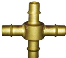
The BCX and the BCXR Series are bite-style cross fittings. The BCXR Series is the reduced version of the BCX Series. These crosses have single sharp barbs to securely hold the tubing from slipping or pulling off. They are excellent fittings for use with Polyurethane or Polyethylene tubing. Made in Brass, Nickel-Plated Brass, or 303 Stainless Steel. Available barb sizes range from 1/16 inch to 3/8 inch.
