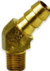
The BHME45 Series is a Forged Brass multi-barbed 45° Elbow with male NPT threads. Flow can be equal or reduced. The temperature range is -40° F to 160° F and the working pressure is 150 psi. Furthermore, the Barstock is optional for the sizes shown below.
