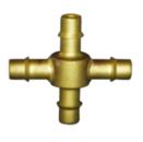
The BCX and the BCXR Series are bite-style cross fittings. The BCXR Series is the reduced version of the BCX Series. These crosses have single sharp barbs to securely hold the tubing from slipping or pulling off. They are excellent fittings for use with Polyurethane or Polyethylene tubing. Made in Brass, Nickel-Plated Brass, or 303 Stainless Steel. Available barb sizes range from 1/16 inch to 3/8 inch.
