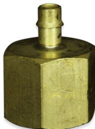
The DFA Series is a Brass female NPT threads-to-bite-style barb adapter. Available in sizes ranging from 1/8 inch to 1/2 inch. This fitting has excellent vibration resistance and requires no clamp. The maximum working pressure is 150 psi and the temperature range is -65° F to 90° F. This fitting can be used in humidifiers, pneumatic systems, and filters.
