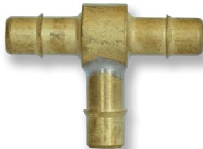
BT Series fittings are available in Brass, Nickel-Plated Brass, 303 Stainless Steel, and 316 Stainless Steel. Designed for use with Polyurethane or Polyethylene tubing for securely holding the tubing from slipping or pulling off. Available barb sizes range from 1/32 inch to 3/4 inch.
