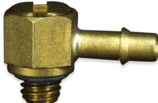
The CAE Series are Brass 10-32 inch UNF by bite-style single barb adjustable fitting with slotted adjustment flush to the surface. Elbow and Tee configurations. Also available in Nickel-Plated.
