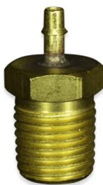
The DMA Series a Brass male NPT thread to ID bite-style barb adapter that works well with Polyethylene tubing. This fitting has excellent vibration resistance and requires no clamp. The maximum working pressure is 150 psi and the temperature range is -65° F to 90° F. Available MNPT thread sizes are 1/16 inch, 1/8 inch, 3/8 inch, 1/4 inch, and 1/2 inch. ID sizes range from .170 inch to .375 inch.
