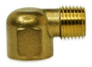
The BSTE Series are 90° Brass Street Elbows, available as both forged and barstock. The barstock fitting is available in a short version. The forged is available as a reducer. Available MNPT and FNPT thread sizes are 1/8 inch, 1/4 inch, 3/8 inch, 1/2 inch, and 3/4 inch. The temperature range is -65° F to 250° F. The operating pressure is 1200 psi. They can be used for grease, fuels, refrigeration and hydraulic applications. They meet ASA, ASME and SAE specifications.
