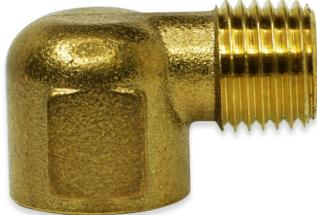
The BSTE Series are 90° Brass Street Elbows, available as both forged and bar stock. The bar stock fitting is available in a short version. The forged is available as a reducer. Available MNPT and FNPT thread sizes are 1/8 inch, 1/4 inch, 3/8 inch, 1/2 inch, and 3/4 inch. The temperature range is -65° F to 250° F. The operating pressure is 1200 psi. They can be used for grease, fuels, refrigeration, and hydraulic applications. They meet ASA, ASME, and SAE specifications.
