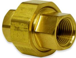
The FXF Series is a Brass female-by-female union. The brass fittings are available in four sizes, the nickel plated in five sizes, as noted below. The maximum operating pressure is 1200 psi and the working temperature range is -65° F to 250° F.
