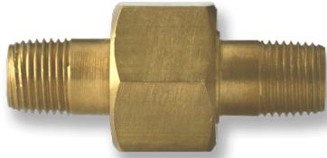
The BXU Series is a Brass male Union. Available male NPT thread sizes are 1/8 inch, 1/4 inch, 3/8 inch, and 1/2 inch. One end of this union is solid with hex nut, the other end can be removed.
