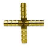
This series of Brass connectors is composed of straight connectors, elbows, tees, and crosses. The working temperature range is  $-40^{\circ}$  F to  $160^{\circ}$  F. The straights, tees, and crosses have equal barb sizes. The elbows are both equal and reducing. These fittings are designed for use with hose clamps.
